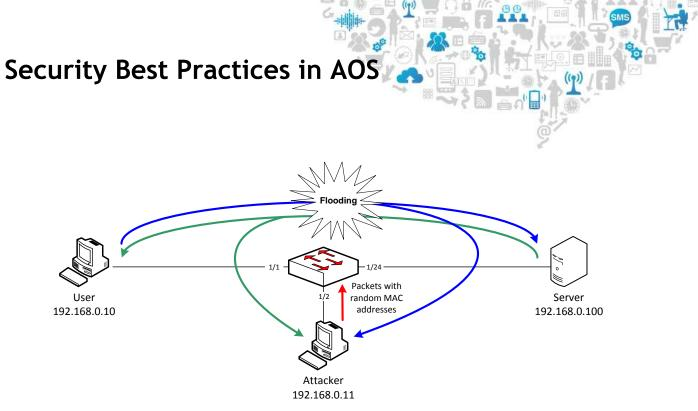
CAM overflows attacks can be mitigated using the Learned Port Security feature (LPS). This feature limits the maximum number of MAC addresses which can be learned on a port, or shuts a port down if this limit is reached.
