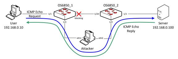
This type of an attack can be prevented using the "qos user-port" feature with BPDU shutdown action:
