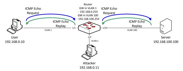
To disable ARP Spoofing protection on an AOS switch use the "ip dos anti-spoofing disabled" command and update "ipni\_arp\_poison\_lrn" variable in dshell:
